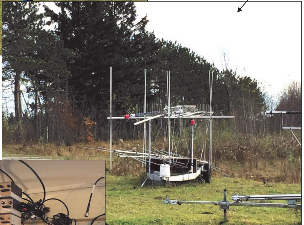
A second 6 meter tower is now down with the two long boom 222 yagi and quagi stored here
